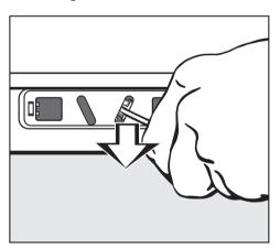
■ Insert a screwdriver into the notch of the right opening and pull downwards. The door will now open.
